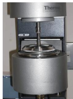
Fig.1 Cone and plate rheometer for shear viscometer
