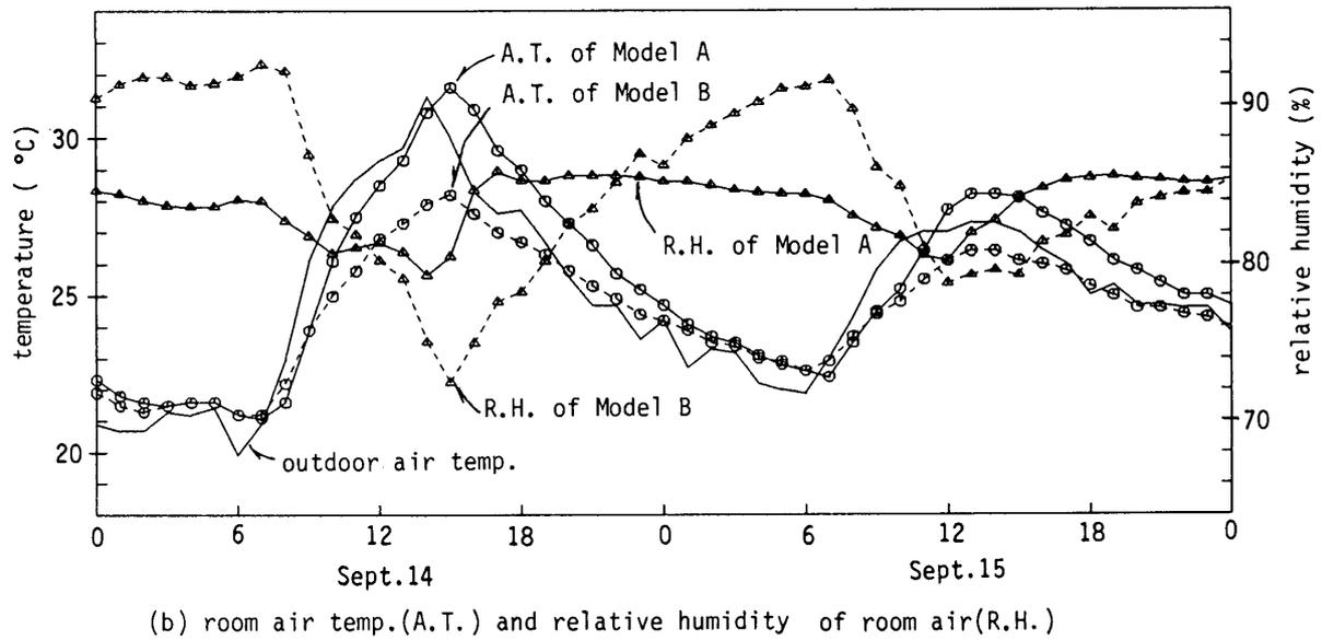
Fig.7 Results of Experiment No.1, all the openings in Model A are closed and Model B is the passive cooling house.
