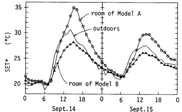
Fig. 10 Fluctuations of the Standard Effective Temperature, SET\*, in Experiment No. 1.
