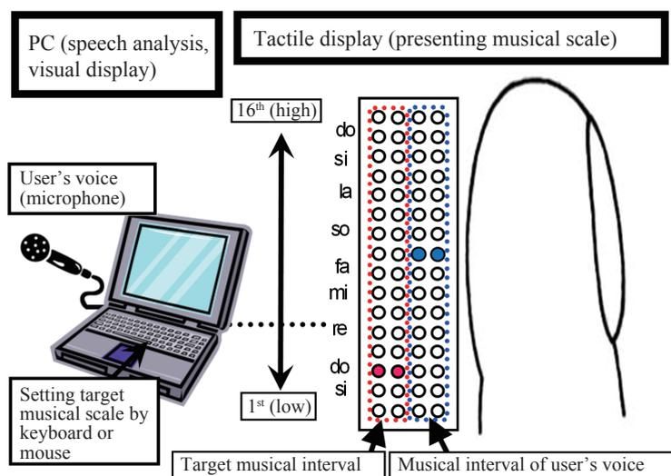
Figure 1. Schematic diagram of the voice pitch control system.
