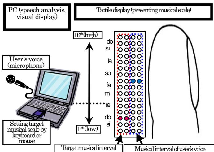
Figure 1. Schematic diagram of voice pitch control system.
